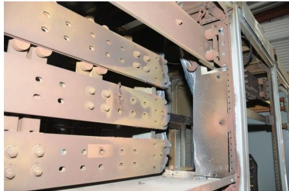
The Plaintiff's experts alleged that the Isolation Barrier was too flimsy to serve its intended purpose of isolating the two sides of the Switchgear. The proposed causation scenario was that the electrician, while positioned in the Load Side Section of the Switchgear, had leaned against the Isolation Barrier, which in turn deflected and contacted the energized phases of the bus bars positioned on the Line Side Section of the Switchgear.
